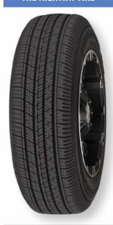
The Forceum Heptagon HT is an all-season tire perfect for navigating the highway. Featuring an asymmetrical tread design, sequential ribs on shoulders, and tread siping, this tire offers excellent traction and handling. The Heptagon HT contains optimal pitch variation as well, which ensures low-noise for a comfortable driving experience.
