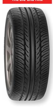
The Forceum D850 is an ultra-high performance passenger tire designed for comfort and wet performance. It features a zig-zag shoulder block pattern to reduce noise and clear water, and a dynamic semi rib block for grip and wet handling. The Forceum D850 also features a continuous center rib, allowing for stability on straight roads.
